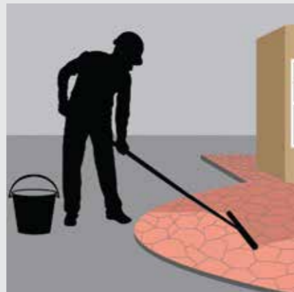
4 Application of Sealant
